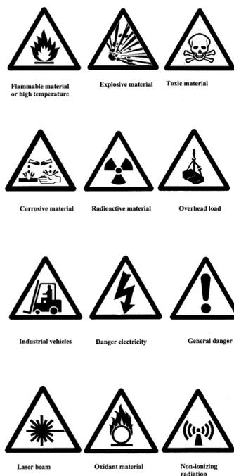
Note—“Flammable material or high temperature” sign in the absence of a specific sign for high temperature
